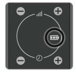
**b** When Revitive is switched off but on charge, the battery indicator icon will constantly scroll during charging; when the battery is full, scrolling will stop.
