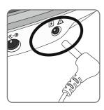
**e** Plug the other end of the Electrode cord into the socket on the side of Revitive.
