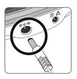
**b** Plug the small end of the power cord into the adapter socket on the side of the device.
